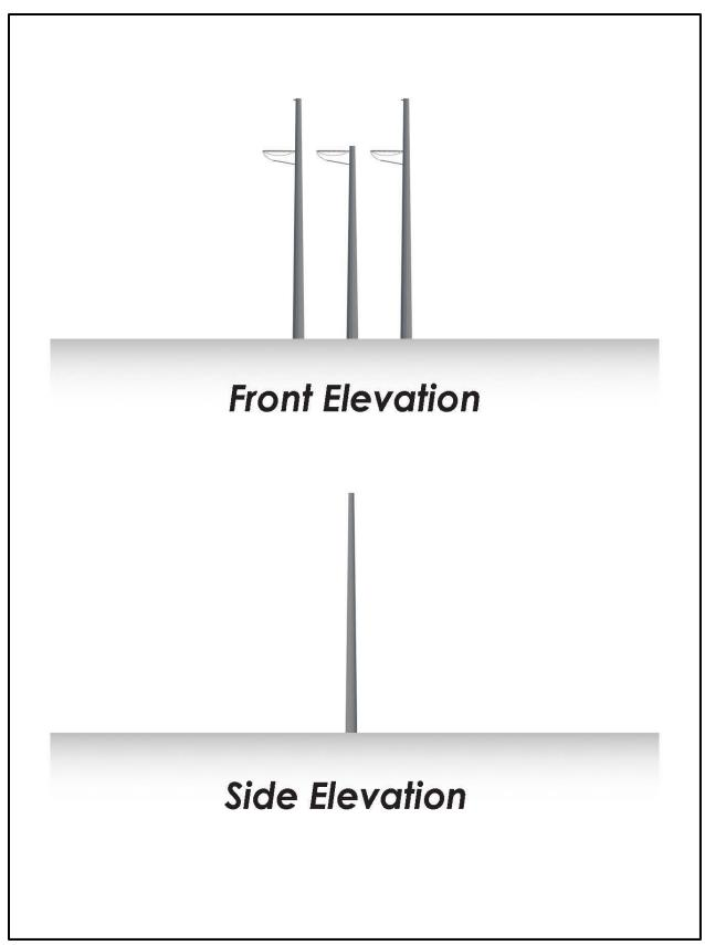
Exhibit G-3. Typical 230kV three-pole dead-end self-supporting monopoles structure.
