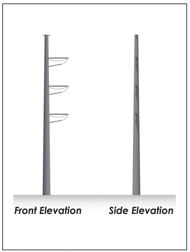
Exhibit G-2. Typical 230kV angle self-supporting monopole structure.
