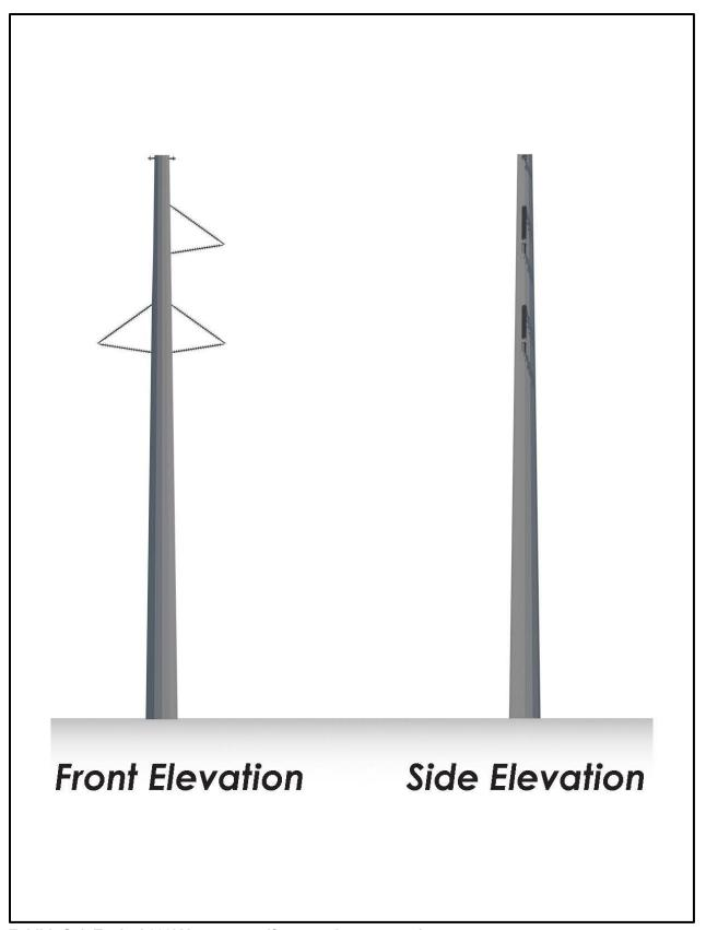
Exhibit G-1. Typical 230kV tangent self-supporting monopole structure.
